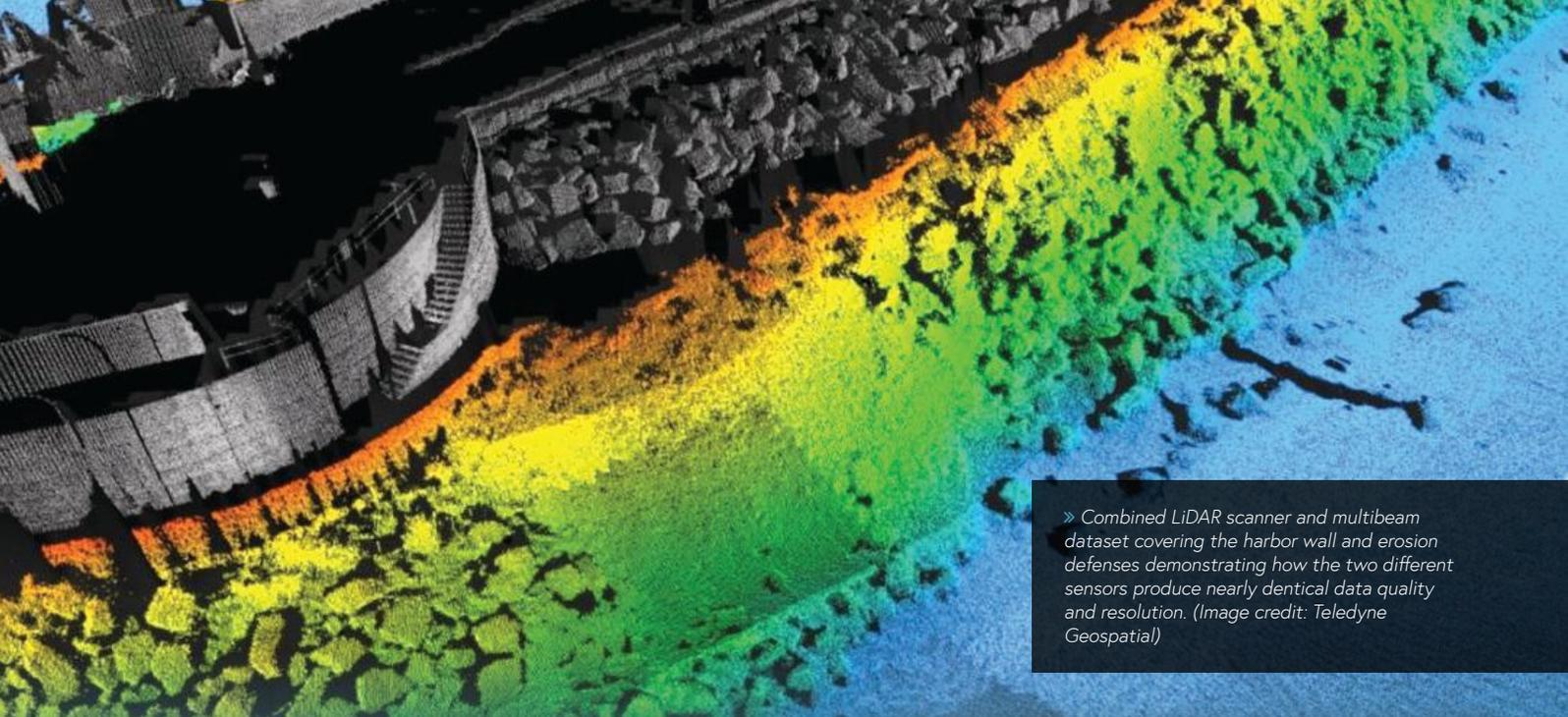
» Combined LiDAR scanner and multibeam dataset covering the harbor wall and erosion defenses demonstrating how the two different sensors produce nearly identical data quality and resolution. (Image credit: Teledyne Geospatial)
