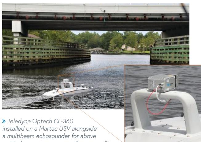
» Teledyne Optech CL-360 installed on a Martac USV alongside a multibeam echosounder for above and below water coverage. (Image credit: Teledyne Geospatial)
